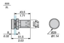
e Support panel thickness: 1 to 6 mm/0.4 to 0.24 in. (metal), 2 to 6 mm/0.8 to 0.24 in. (plastic).
